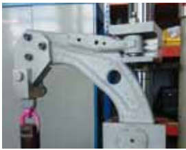
Fatigue life of a welded car wishbone Validation of self-heating modeling results taking in account welding process effect
